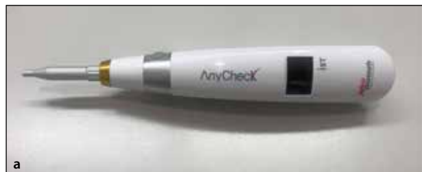
Fig 2 (a) Implant stability measuring device using a damping capacity assessment. (b) This device measures a contact time with a target from the reciprocating metal tapping rod.
